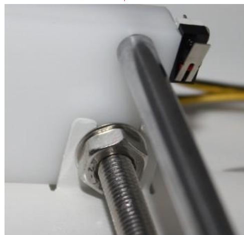
The Y-axis module screw cap after the alignment with the U-shaped slot fixed with the back end of the batter board
