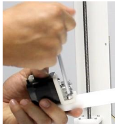
Use a socket head wrench to tighten the screws: M6*10-2pcs
