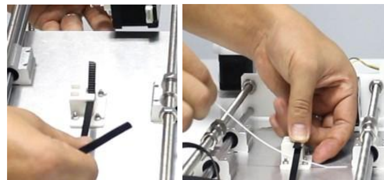
Imbed the synchronous belt into the belt clip and turn back the synchronous belt and tighten it with a ribbon.
