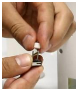
Put the screw M2*16-2pcs through the limit switch and sheathe the 5mm shoot-through column
