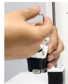
Use a socket head wrench to tighten the screws M3*12-3 pcs
