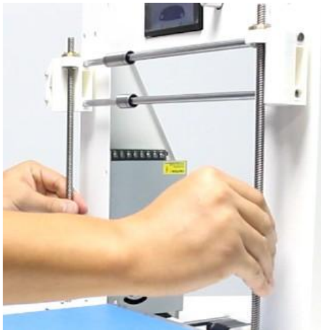
Screw the slick rod with both hands to see whether it moves smoothly. If it doesn't move smoothly, it is required to move the X-axis motor seat or driven seat inwardly a certain distance until the slick rod can be smoothly screwed. Then install the \phi 8 \times 321-2 to the Z-axis motor mounting holes.
