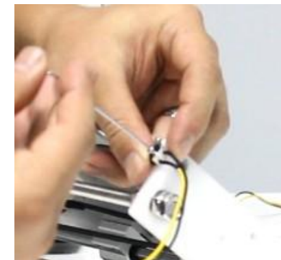
The shrapnel of the limit switch is toward the box-type bearings. Use the socket head wrench to tighten the screws M2*10-2pcs
