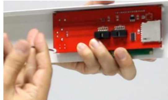
Screw the lcd display with the plastic screws by allen wrench(4* M3*10 screw)
