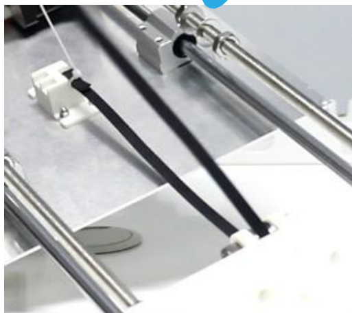
The side with synchronous teeth round passing the bearing and synchronous wheel
