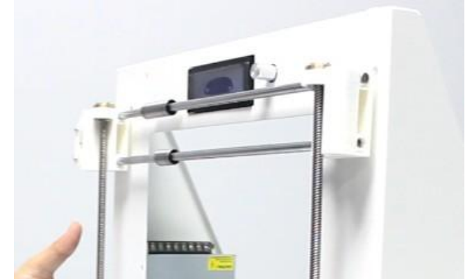
While installing, avoid the knob of the display screen and align the whole of the T-shaped nut.
